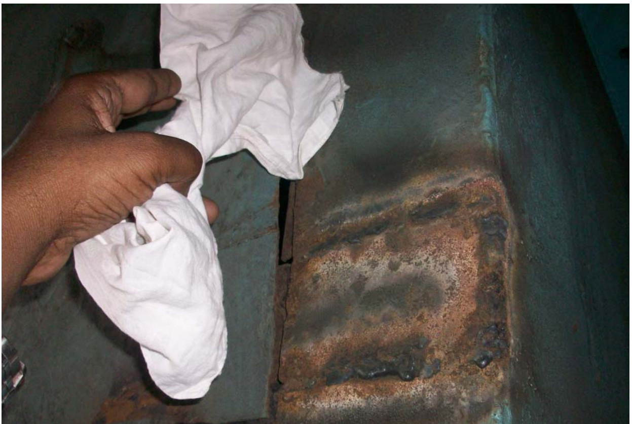
Photo 5: Suction effect seen at feeder discharge chute to mixing nozzles.
