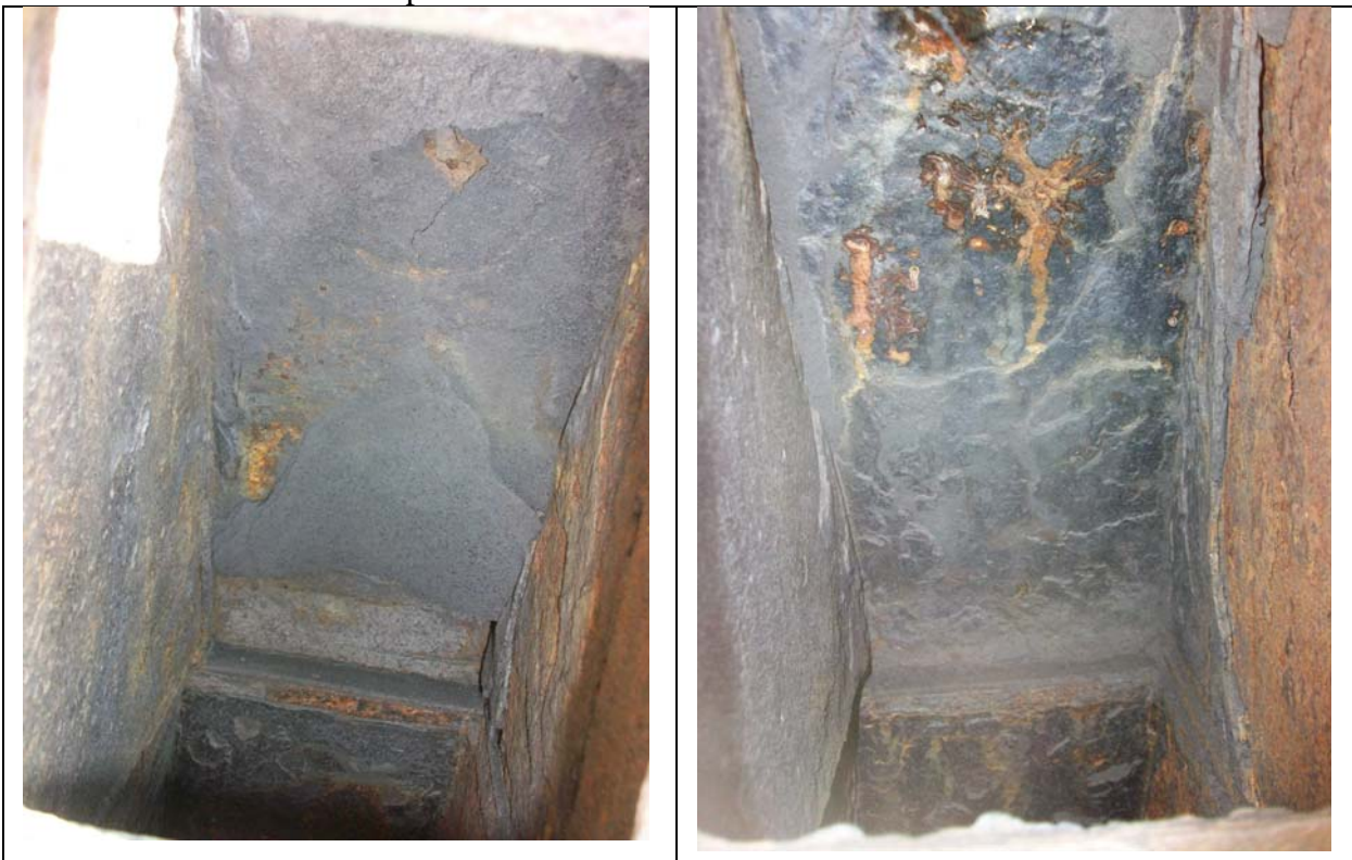
Photo 16 & 17: The above were snaps from old mixing nozzle inlet chutes. The coal dust was seen sticking inside the mixing nozzle inlet chute. This must have occurred more in the old mixing nozzles, as they were always on positive pressure at throat.
