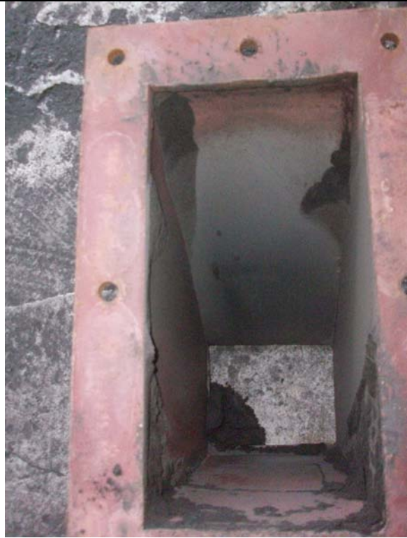
Photo 12 & 13: The effect of tack / stitch weld was seen very well in this chute, which was dismantled from position in boiler no2 during the visit. The weld beads had acted as nuclei for dust build up. Ideally the weld should not be present in the coal path.
